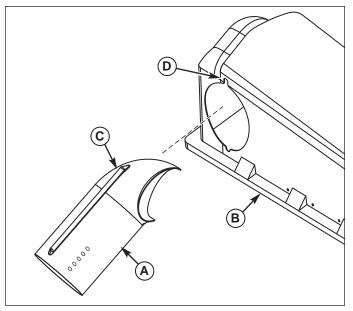
Figure 13. Install Upper Tube to Cover
